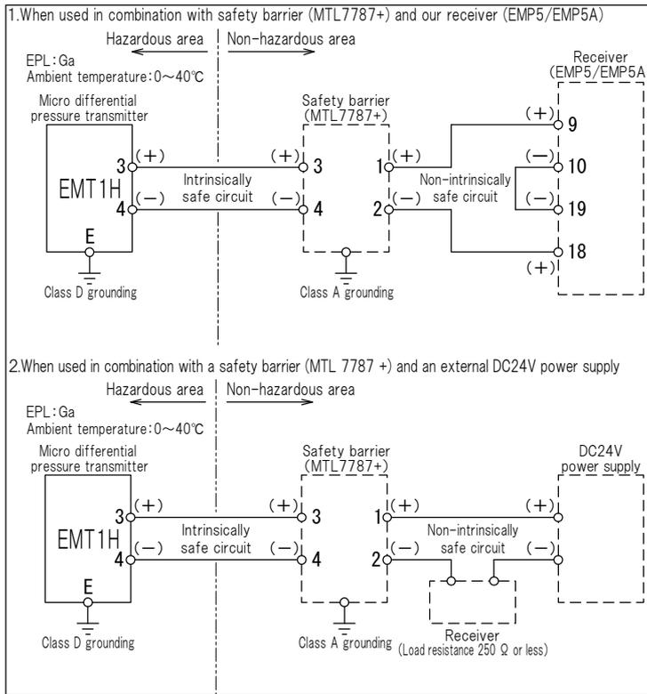
• Since our receiving instrument incorporates the DC power supply circuit for micro differential pressure transmitter, no separately-installed DC power supply is required.
